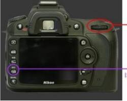
Rear Wheel: Used to control Shutter Speed
